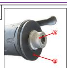
OEM bar-end weight removed
