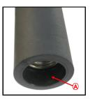
OEM Bar-end weight removed
