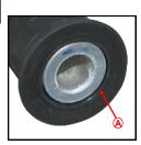
OEM bar-end weight removed, exposing the plastic throttle sleeve
